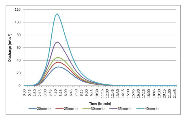
Fig 26: Runoff hydrographs for precipitations with triangularly distributed intensities
