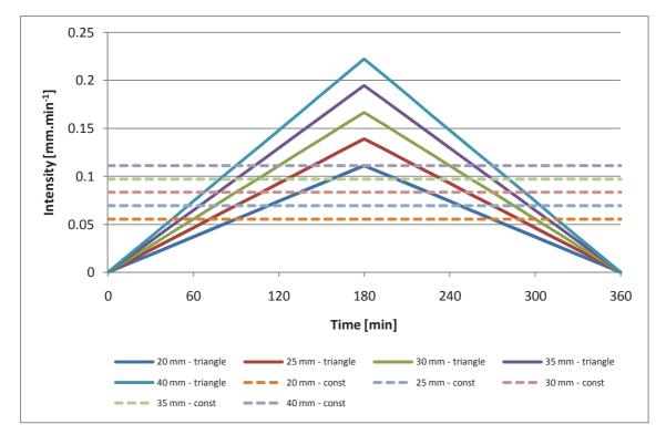
Fig 25: Distribution of precipitation intensities used for flood simulations
