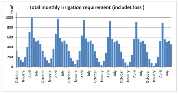
Fig 28: Graphic description of irrigation water demand including losses according to different irrigation technologies
