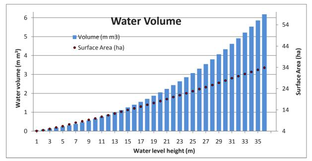
Fig 29: Relationship between water depth and volume in planned reservoir
