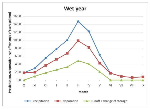
Fig 23: Water balance in wet year
