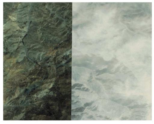
Fig 15: Data errors – orthophoto – damaged stripe with clouds
