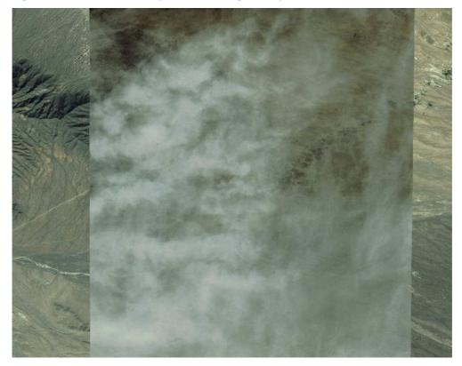
Fig 16: Data errors – orthophoto – damaged data stripe
