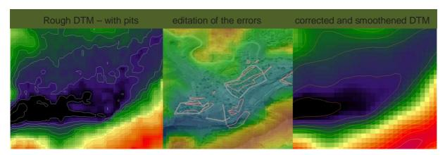
Fig 8: Preparation and editing of digital elevation model - removal of wrongly evaluated places
