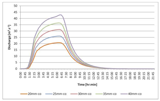
Fig 27: Runoff hydrographs for precipitations with constant intensities
