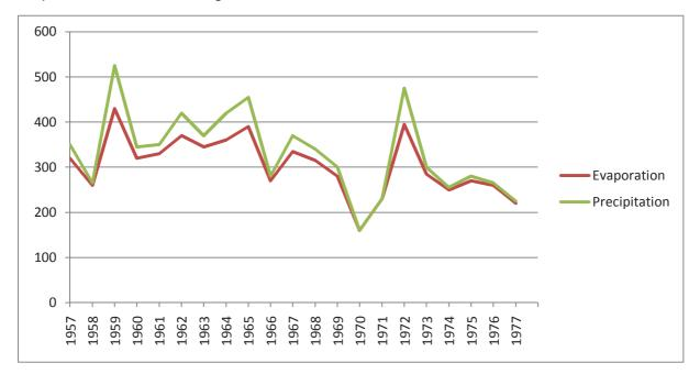
Fig 19: Annual values of measured precipitation totals and total annual evaporation calculated after Turc in period from 1957 to 1977; taken from (Tünnermeier, 2005)
